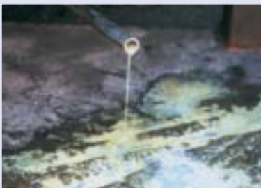
Unwanted Abrasive Sludge
